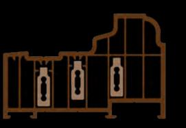
window frames are typically 3 or 5 chambers and are usually 70mm wide, Residence 9 has 9 chambers and is 100mm wide, resulting in superior thermal, acoustic, strength and security performances.
